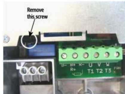
Fig. 5.g – Changing of EMC protection class, MF4 (left) and MF5 (right).
