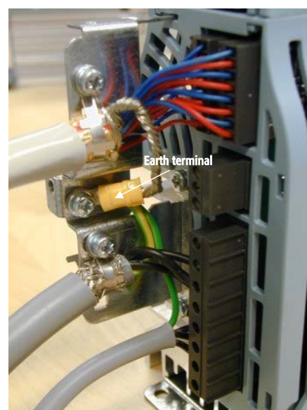
Figure 6.i. Cable installation for MF3
