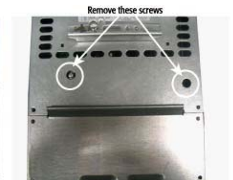
Figure 5.h - Changing of EMC protection class, MF6
