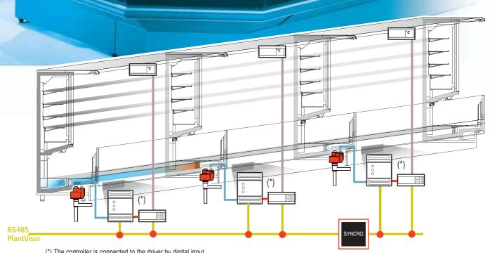
(\*) The controller is connected to the driver by digital input.
