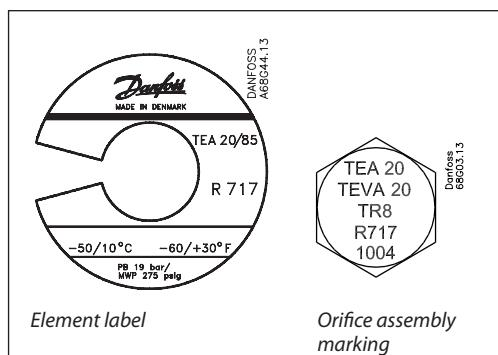
The thermostatic element has a white label attached to its top. The colour refers to the refrigerant for which the valve is designed: R 717 ( $\text{NH}_3$ ).
