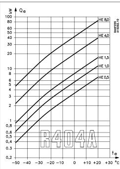
Precise heat exchanger sizing can be obtained from the curves which show plant capacity  $Q_{\rm e}$  for R22, R134a and R404A depending on evaporating temperature  $t_{\rm e}$ .
