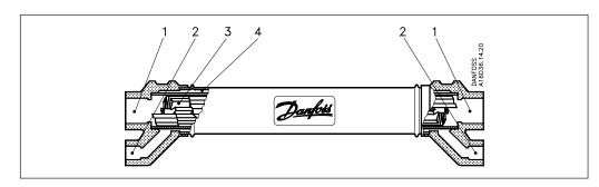
Offset fin sections are built into the inner chamber (3) and result in turbulent gas flow with minimum flow resistance.
