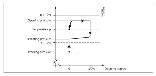
BSV is designed as a standard safety relief valve (DIN 3320) which are recommended for refrigeration plants. On a rise in pressure above the set pressure, the safety relief valve will initially start opening slightly, to minimise the outlet of refrigerant. If the pressure continues to increase, the valve will open fully. The safety relief valve will be fully open before the pressure is 10% higher than set pressure, and fully closed before the pressure is 10% below set pressure.
